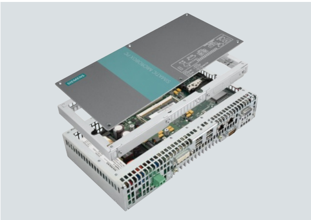
SIMATIC IPC427C with expansion frame
