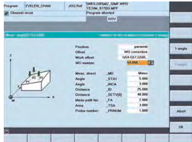
Measuring cycles Example: 2-angle measurement for determining the position of a plane in space
