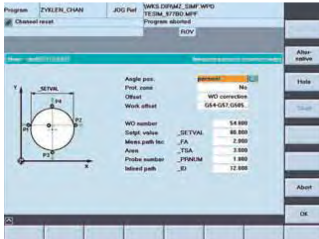
Measuring cycles Example: Measuring a shaft
