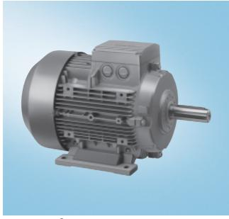
The SIEMOSYN® 1FU8 motors are permanent magnet excited synchronous motors with a squirrel-cage winding for asynchronous self-starting. They can be operated as constant-speed drives on the mains, or as variable-speed single-motor or multimotor drives on the inverter.
