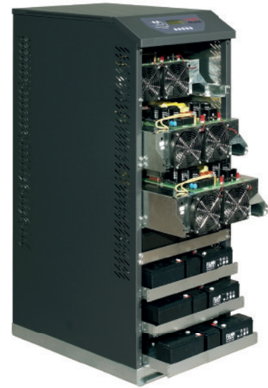
UPS electronics (modular construction / power modules)
